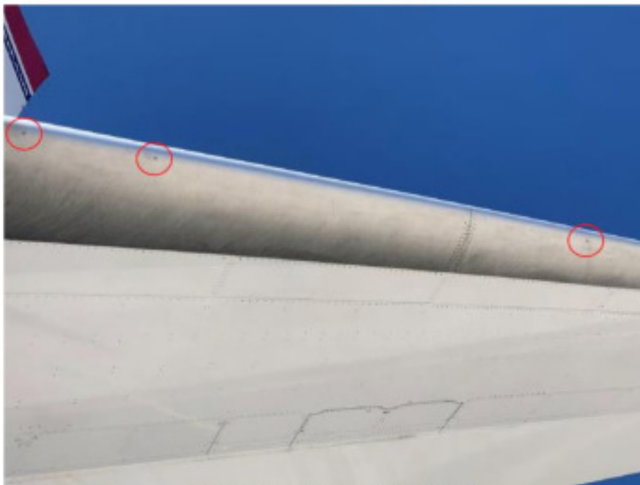
Picture 8: aircraft damage, horizontal stabilizer.
