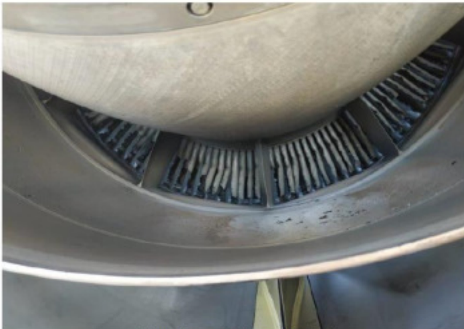
Picture 3: external evidence of left engine damage.
