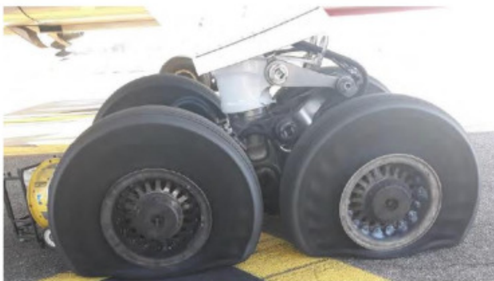
Picture 10: deflated left landing gear tires.
