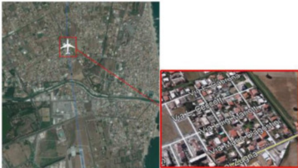
Figure 3: position of the aircraft at the activation of the FDR discrete parameter "Eng1_Vib_Warn"; details of the streets around that area, where debris from the left engine were collected.
